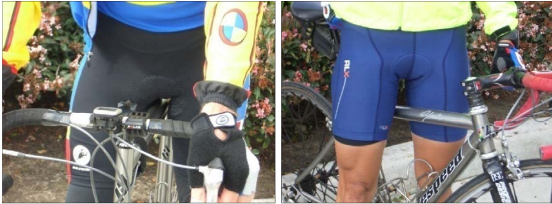
Figure 2. Road bicycle frame size. Left: Allow at least 1 inch of clearance between the top tube and your crotch. Right: Compact road frames, like mountain bikes, will allow even more room.
